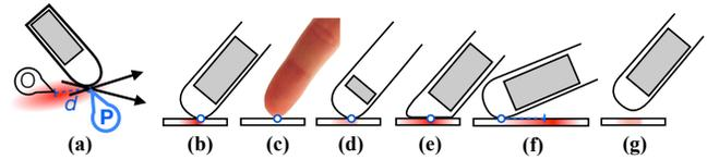
Figure 6. Sensing with touchscreens. Red: Magnetic field intensity. (a) Overview, (b) stylus event, (c) touch event, (d) different styli, (e) various pressures, (f) different tilt angles, and (g) hover.
