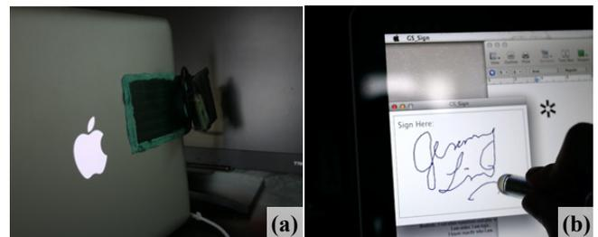
Figure 16. (a) Attaching sensor board to back of laptop monitor, and (b) taking a note.
