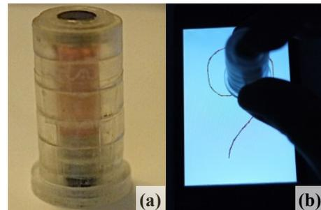
Figure 9. (a) Apparatus for testing. An acrylic case is used to keep a stylus perpendicular to the sensor board. (b) Drawing an arbitrary curve for sampling; the connected black and red points represent positions P and O, respectively.
