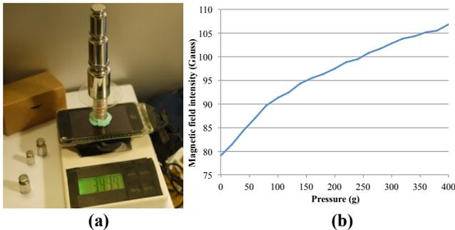
Figure 11. (a) Experimental apparatus. (b) Results of magnetic field intensity using 0 to 400g weights.
